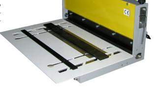
The device is equipped with a unique movable table plate. It allows for performing six different creases without resetting the machine.
