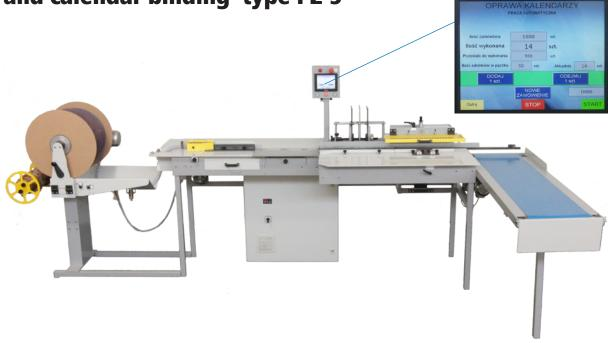
Both large and small quantities can be bound, as choosing the correct setting is fast and simple. Thanks to the touch screen control panel which displays successive steps of the process, the operator is able to set the machine correctly and very fast. There is no need to change any parts for various settings. When the machine is in operation, the most important information is presented on the display panel:
